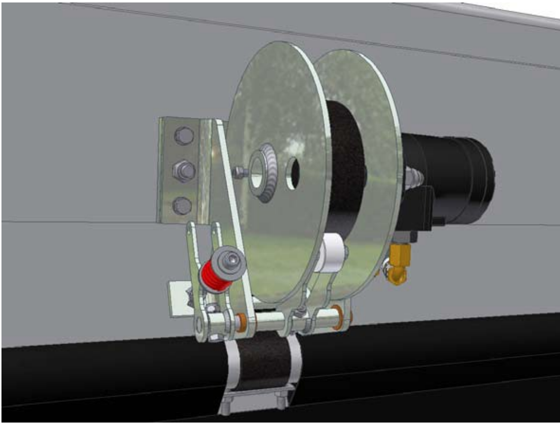
Figure 2: Winch mounted at top of front wall.
